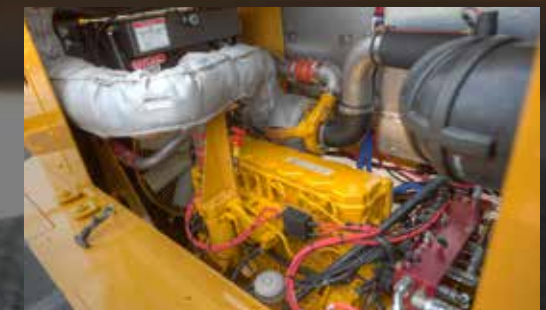
QSB-6.7 Liter Cummins Electronic Turbocharged Diesel Engine
